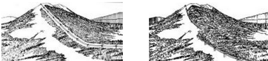
Figure 8.21: New disturbance should be avoided and the natural lines in the landscape should be followed. (Source: US-BLM, 2009)
